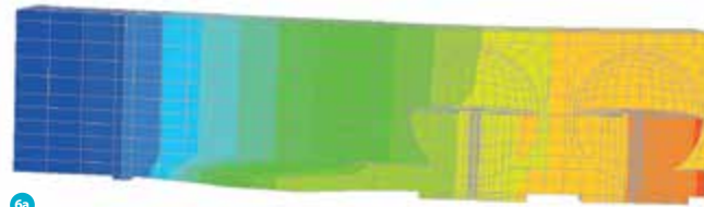
v2a load-step 153, load-factor 150.00, LC2_load displacements TD+Z min: -12.2 mm max: 2.8 mm
